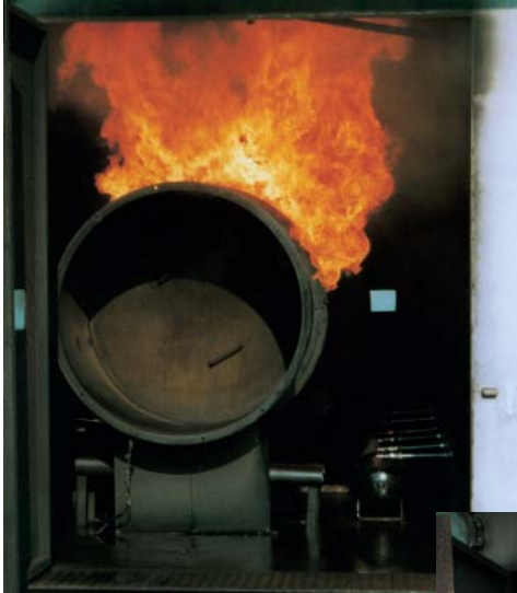
Test fire: Full fire on an insulation soaked with gas oil
